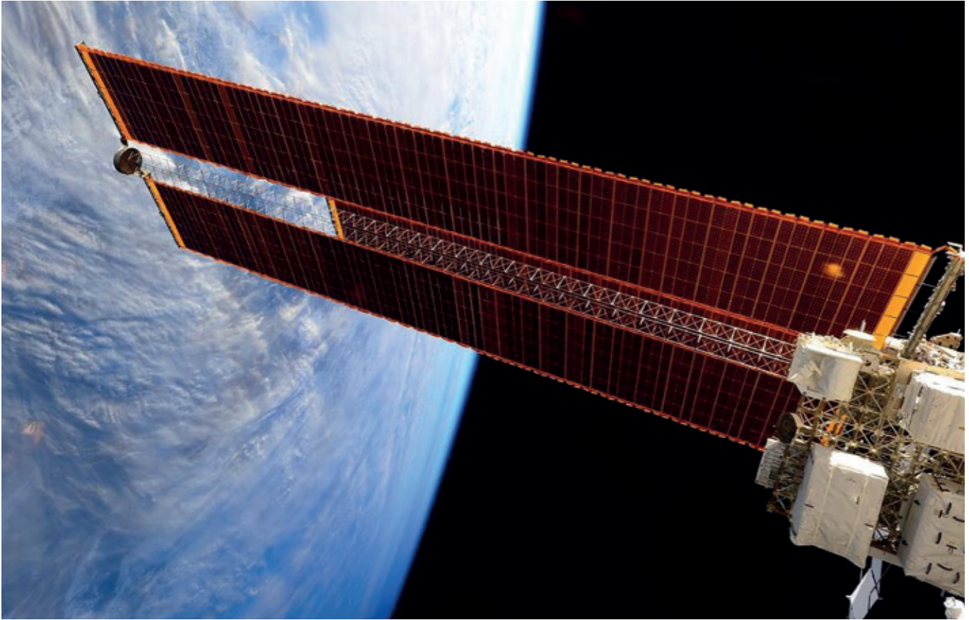
A single section of the massive solar arrays aboard the ISS
