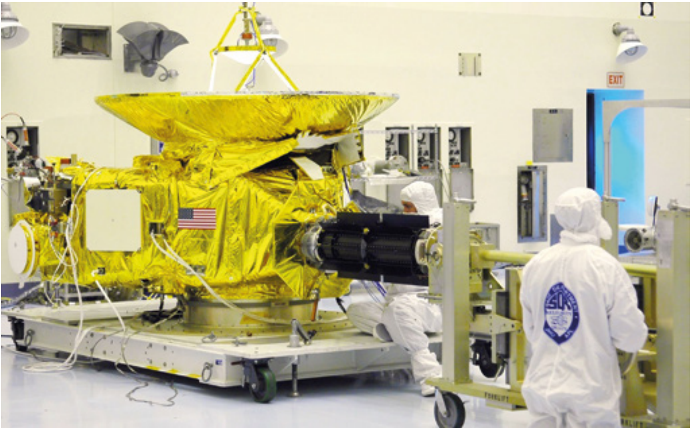
Figure 2 NASA workers installing the RTG onto the New Horizons spacecraft prior to launch
